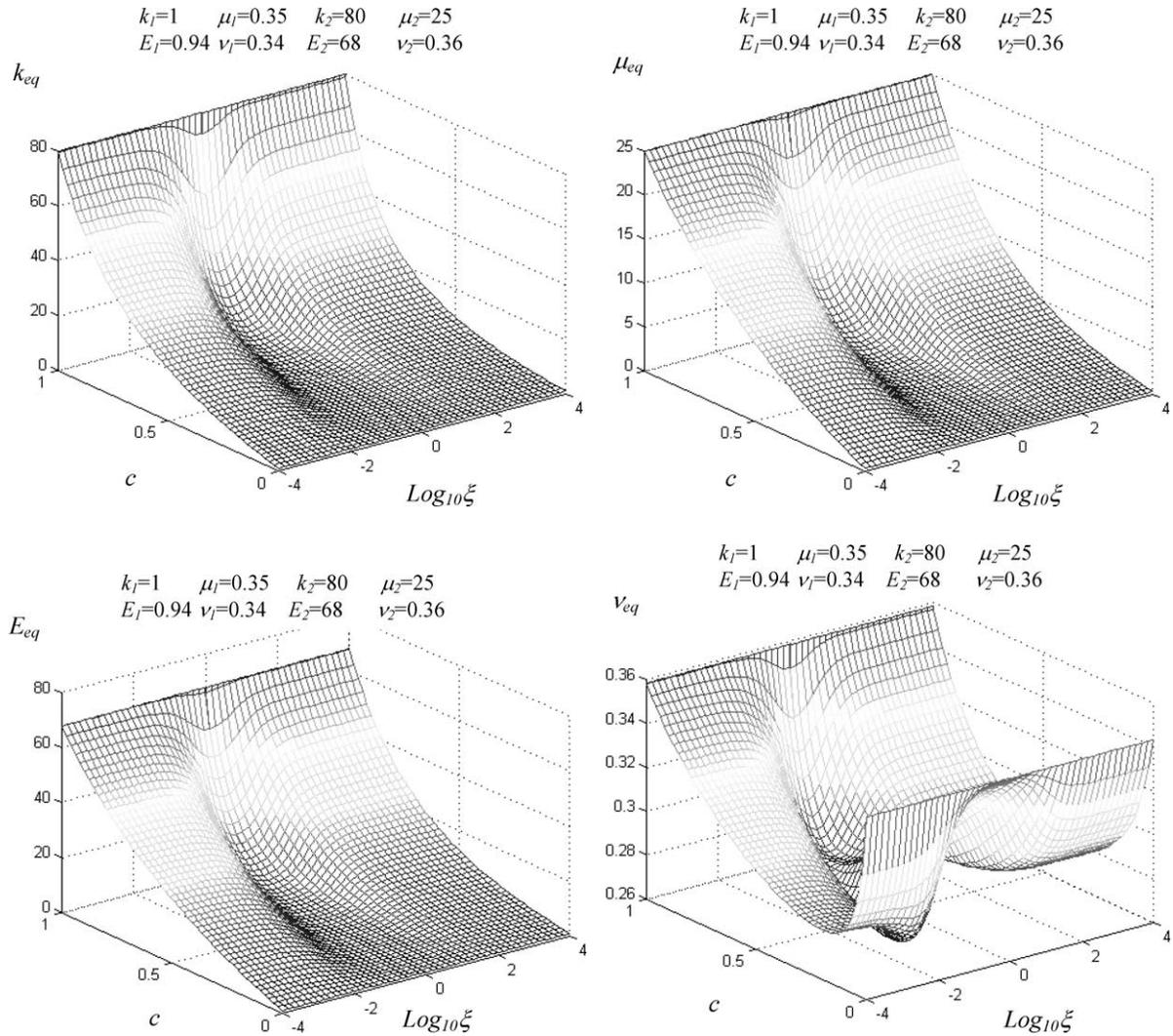
Fig. 4. Results obtained by means of the differential scheme (Eq. (30)) applied to a dispersion of ellipsoids of rotation. The elastic constants (bulk, shear, Young and Poisson) are plotted versus the eccentricity  $\xi$  (ratio between the longer and the shorter axis of the embedded ellipsoids) and the volume fraction  $c$  with the same assumptions used in Fig. 3 in order to draw a comparison between the theories.
