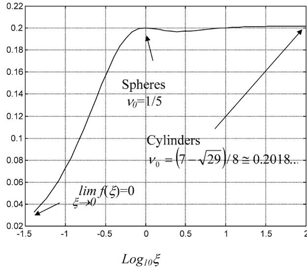
Fig. 7. Universal behaviour of the Poisson ratio for porous materials with high value of the volume fraction (porosity). When  $c \rightarrow 1$  the Poisson ratio depends only on the eccentricity  $\xi$  (ratio between the longer and the shorter axis of the embedded ellipsoids) and not on the matrix elastic properties, as shown in this plot. Characteristic values for spheres and cylinders are clearly evidenced.
