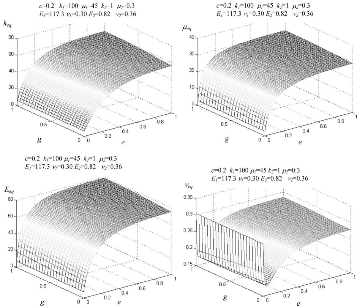
Fig. 2. Effective elastic response for a given dispersion versus the eccentricities  $e$  and  $g$  of the embedded inclusions (ellipsoids with axes  $a_1, a_2, a_3$  with  $a_1 > a_2 > a_3 > 0$ . Eccentricities:  $0 < e = a_3/a_2 < 1$  and  $0 < g = a_2/a_1 < 1$ ). Bulk, shear, Young and Poisson constants have been computed with the theory for diluted dispersions (Eq. (16)) with the indicated assumptions.
