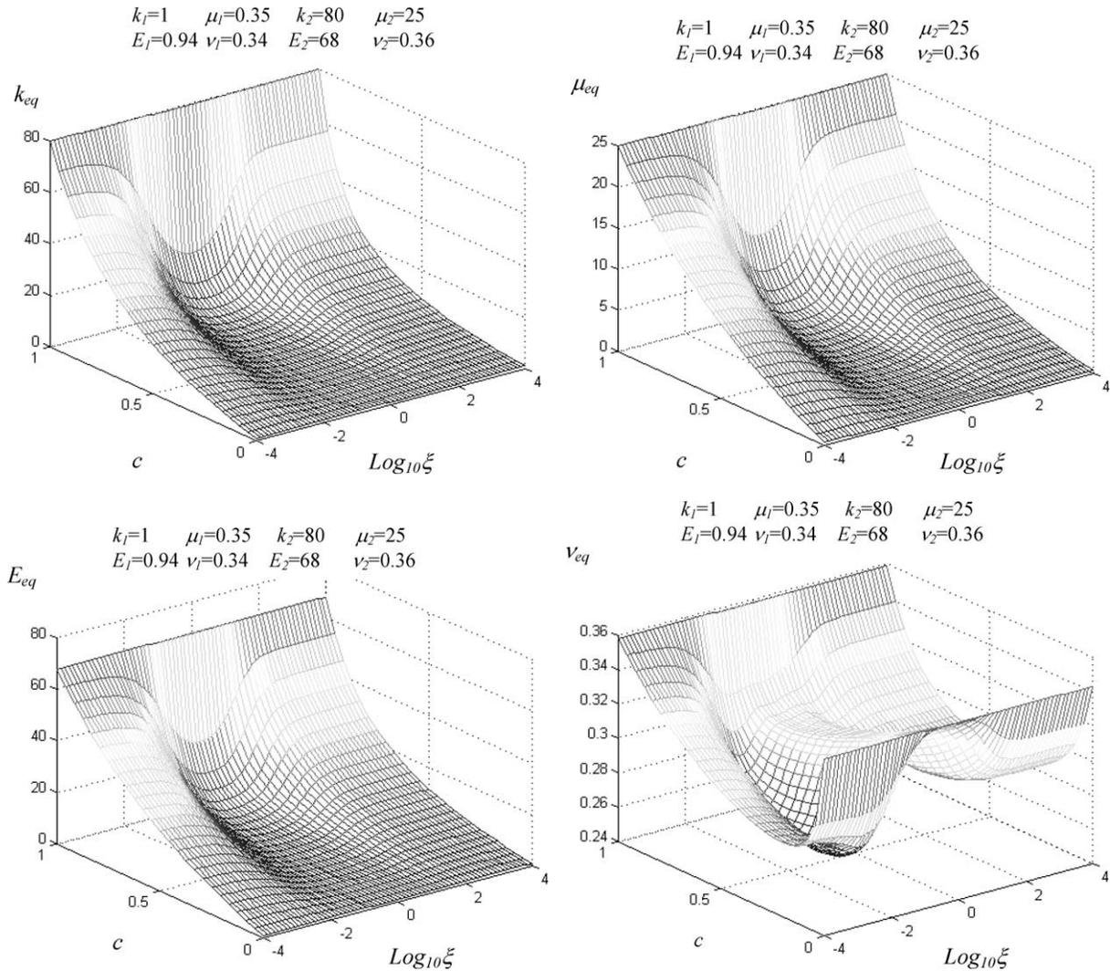
Fig. 3. Results obtained for a mixture of ellipsoids of rotation described by the first procedure (Eq. (16)), holding on for very diluted dispersions. The elastic moduli (bulk, shear, Young and Poisson constants) are shown versus the eccentricity  $\xi$  (ratio between the longer and the shorter axis of the embedded ellipsoids) and the volume fraction  $c$  of the inclusions.
