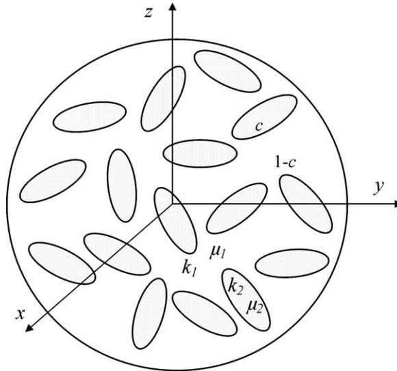
Fig. 1. Structure of a dispersion of randomly oriented ellipsoids. The external surface of the mixture is, e.g., a sphere, which contains all the inclusions. The two-phase material is described by the elastic response of each phase, by the volume fraction of the inclusions and by the characteristic eccentricities of the embedded particles.
