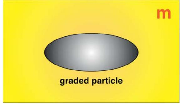
**Fig. 2.** Functionally graded inclusion with arbitrary permittivity profile  $\epsilon(\xi)$  for  $-a_{s_3}^2 < \xi < 0$ .
