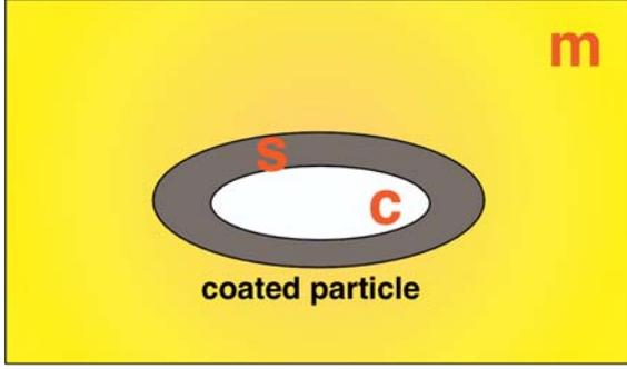
**Fig. 1.** Coated dielectric ellipsoidal particle with isotropic external shell ( $s$ ) and internal anisotropic core ( $c$ ) embedded into a given isotropic matrix ( $m$ ).
