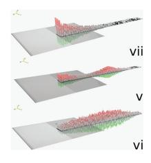
Surface phonon cavity formed by the placement of a defect of a single domain within periodic domain inversion of single crystal piezoelectric lithium niobate exhibiting surface phononic bandgap through the phonon-polariton coupling is introduced. It is shown that the proposed cavity can exhibit entrapment of phonon-polariton, indicated by the simultaneous localization of both surface phonons and the electric within the defect.
